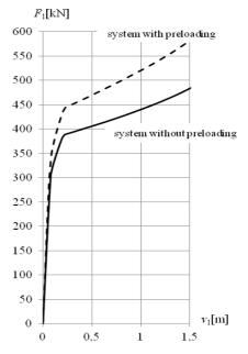
Fig. 8. Load  $F_1$  versus displacement  $v_1$  diagram for the viaduct
