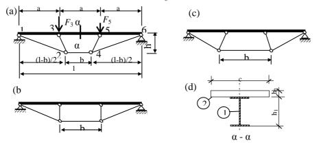
Fig. 1. Scheme with loading of the rod system: (a) b < 1/3; (b) b = 1/3; (c) b > 1/3
