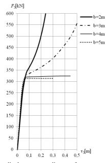
Fig. 2. Load  $F_3$  versus displacement  $v_3$  diagram for system without preloading ( $F_5$ =0)
